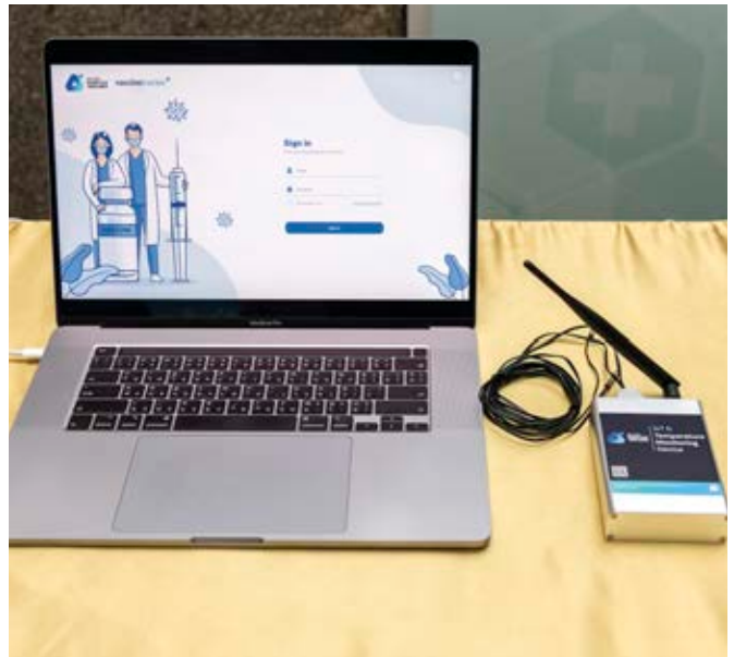
| IoT cold chain monitoring and alert system for COVID-19 vaccine storage
