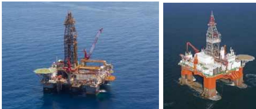
Fig. 7. Example of semi-submersible rig (left picture: ballasted; right picture: deballasted)
