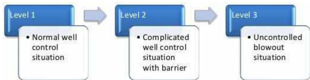
Fig. 47. Levels of Incident during blowout
